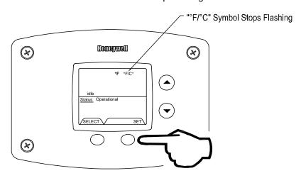
Step 5: Pressing "Select" button will return display to setpoint in format selected (°F or °C) immediately
